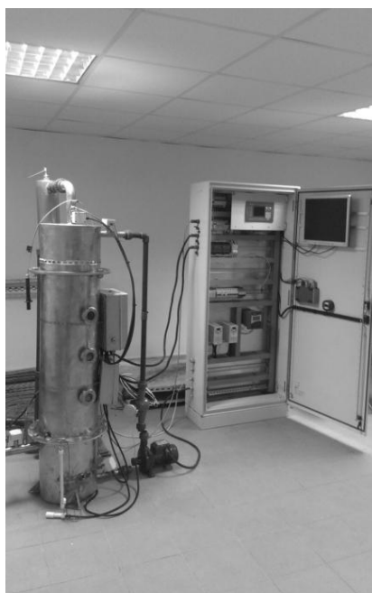
Figure 2: Experimental setup including the bioreactor and cabinet with controls and measuring equipment. Not shown: computer-assisted data logging system
