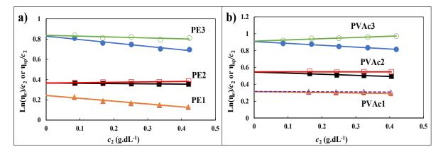
Figure 1. Huggins and Kraemer plots of PE – p-xylene systems at 75 °C (a) and PVAc – methanol systems at 53 °C (b)
