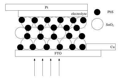
Figure 2: Assembly of the solar battery
