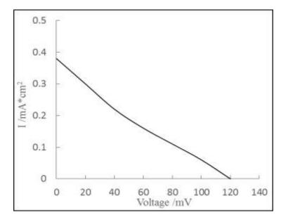
Figure 4: The I-V curve of SnO2 sensitized by PbS quantum dot
