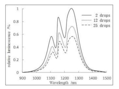
Figure 3: Effect of different drops of SnO2 nanoparticle on the luminescence of PbS quantun dots
