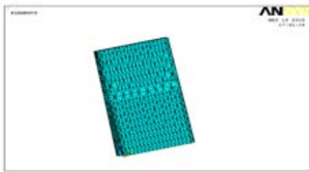
Figure 3: Plate type multi tube wet exhaust chimney mechanical model (before opening holes)
