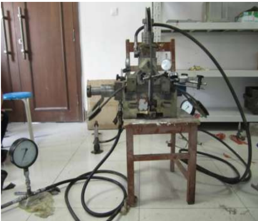
Figure 1: Medium shear test device
