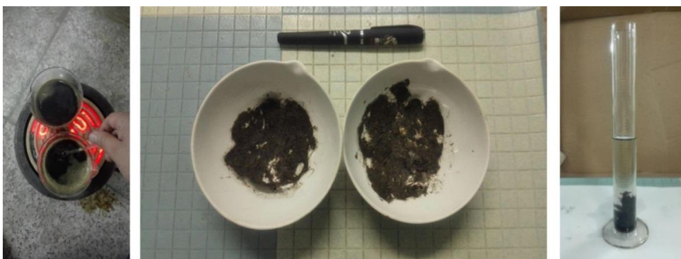
Figure 2: The separation process of plant residues and soil particles
