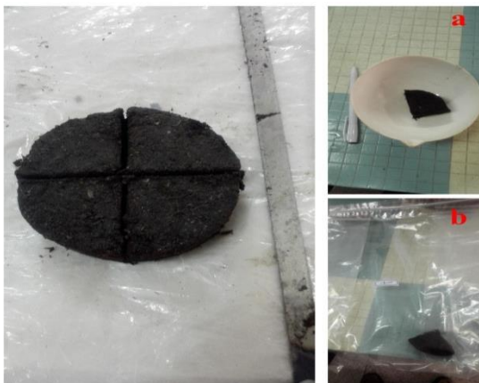
Figure 1: The quartering preparation of turfy soil specimens
