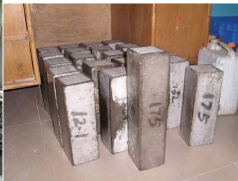
(b) Concrete sample with sealing wax on surface
