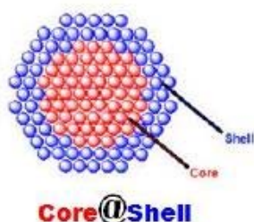
Figure 1: A schematic illustration of core-shell structure
