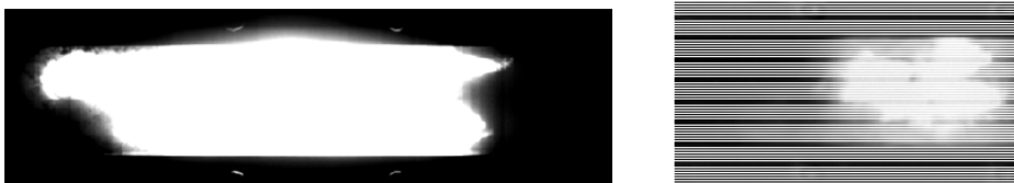
Figure 3: Flame radiation for 30 \text{ } \% wt. Mg/C mixture (left) and for pure lycopodium powder (right) by way of comparison. Dust concentration = 750 \text{ g.m}^{-3} , Ignition energy = 100 \text{ J} , t_v = 60 \text{ ms} .
