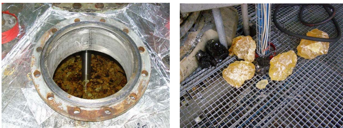
Figure 7: View through the open manhole of the reactor after the incident, showing massive polymerization (left) Pieces of Polymer from the reactor (right)
