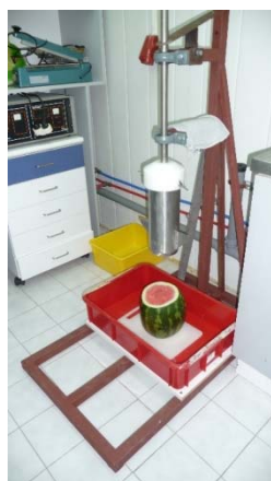
Figure 2. Full size (300 mm long and 120 mm in diameter) of puncture cutter test in construction in vertical operation.
