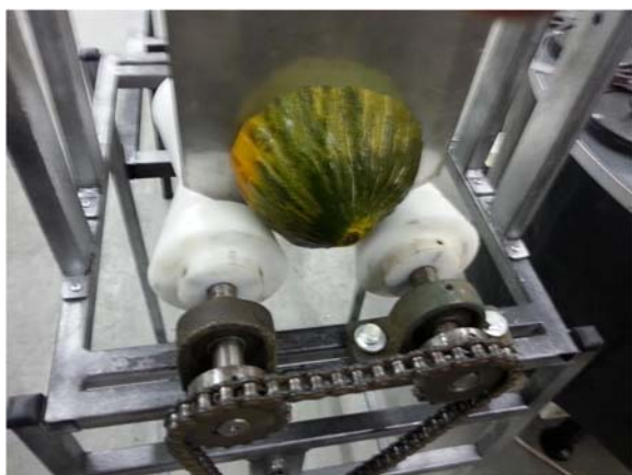
Figure 5. Prototype of edge cutting blades system.
