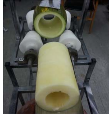
Figure 9 b. The second melon for removing out hollowed cylinder of fresh cut flesh.
