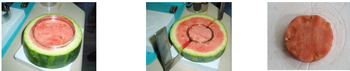
Figure 1. Mechanical cutting and puncture tests based on smooth and perforated steel tubes.
