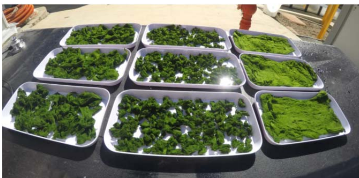
Figure 1: Dewatered and prepared triplicate algae samples prior to solar drying. From L to R: 3x5cm torn samples, 2x2cm cut samples, sheet samples.
