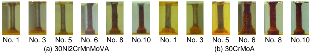
Figure 1: Photos of stress corrosion after 3 days
