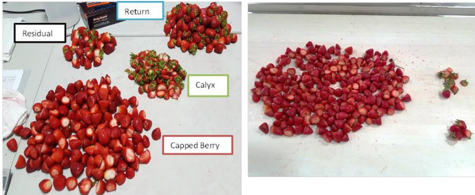
Figure 6. Initial test results: Left: the photo of the spring live demo result. Random samples are taken out from the output conveyor and manually sorted for analysis. Right: Decap output tested during Fall Trial that minimized the calyx and residual elements.
