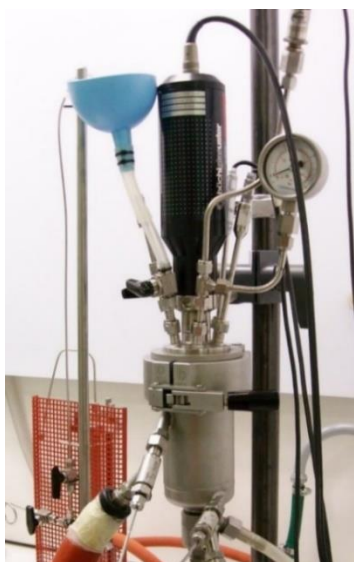
Figure 1. Calorimetric reactor by BüchiGlasUster used for the experiments.
