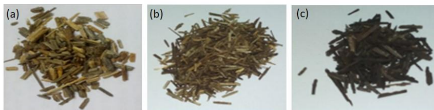
Figure 1: Appearances of the raw and torrefied OPF: (a) Raw biomass (b) Torrefied at 240 °C (c) Torrefied at 300 °C
