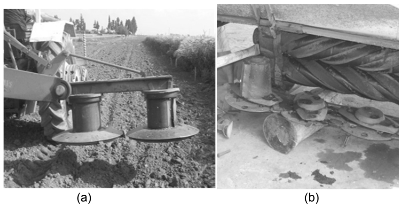
Figure 2. Mower (a) and disc mower with conditioner (b)
