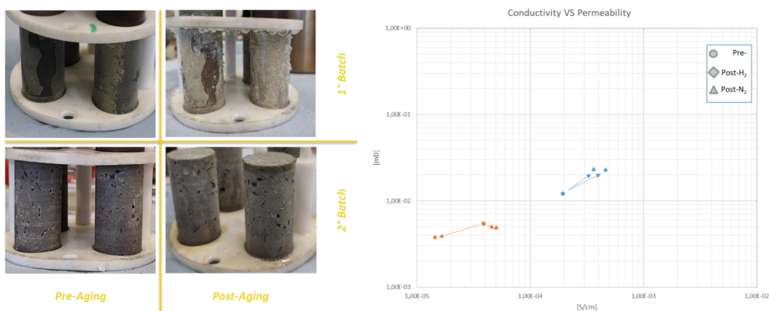
Figure 6a (on left) – Visually unaltered samples after exposure to hydrogen
