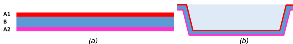
Figure 4: Scheme of the A-B-A structure on the sheet (a) and on the final thermoformed trays (b) as reported in the developed spreadsheet
