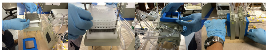
Figure 2: Cement-Structured Zeolite (CSZ) membrane stacking in the ED desalination system
