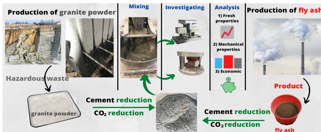
Figure 1: Production of cementitious materials with the synergistic addition of granite powder waste and fly ash
