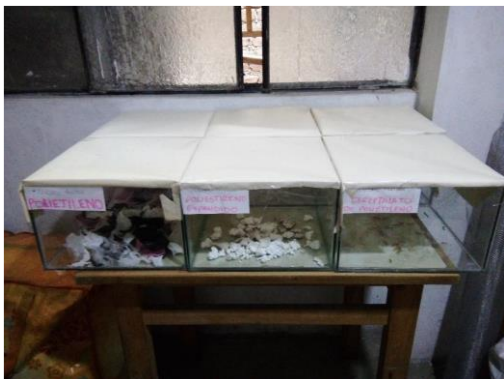
Figure 3: Experimental environment for polymer biodegradation with larvae of Tenebrio molitor and Galleria mellonella
