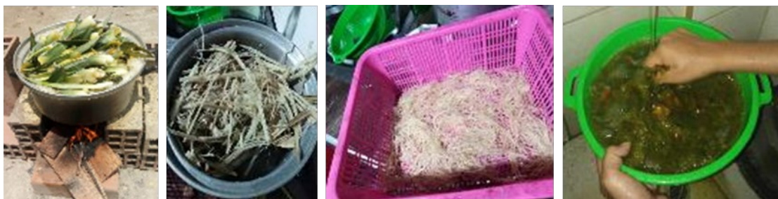
Figure 2: Washing and cooking process of pineapple bud and sugarcane bagasse fibers
