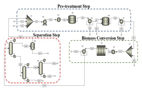
Figure 1: Process flow diagram of 5-hydroxymethylfurfural production using sugarcane bagasse as raw material.
