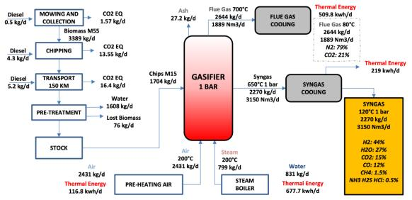
Figure 2 Gasification supply chain. M55 means a humidity percentage of 55% and the syngas composition is given in massif percentage.
