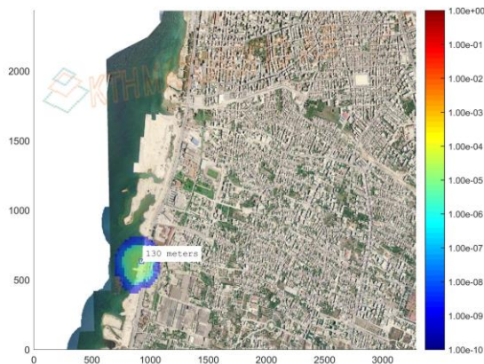
Figure 2: Iso-risk curves for the ship to ship bunkering (Individual risk equal to 10^{-6}/\text{yr} at 130m from the bunkering)
