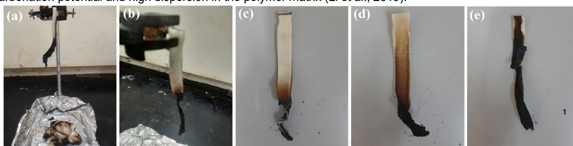
Figure 3: Digital pictures of the UL-94 test for RPUF (a) pure RPUF, (b) RPUF/IFR a 1, (c) RPUF/IFR a 2, (d) RPUF/IFR b 1, and (e) RPUF/IFR b 2.
