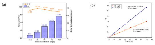
Figure 3: (a) Effect of initial MB concentration, (b) the data fitted to pseudo-second-order models
