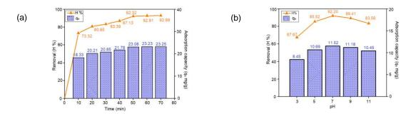
Figure 2: Effect of (a) contact time, (b) pH on adsorption capacity of the CFs aerogel
