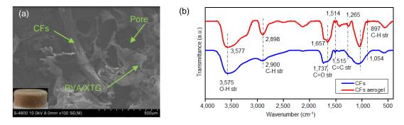
Figure 1: (a) FE-SEM images, (b) FTIR spectra of pretreated CFs and CFs aerogel
