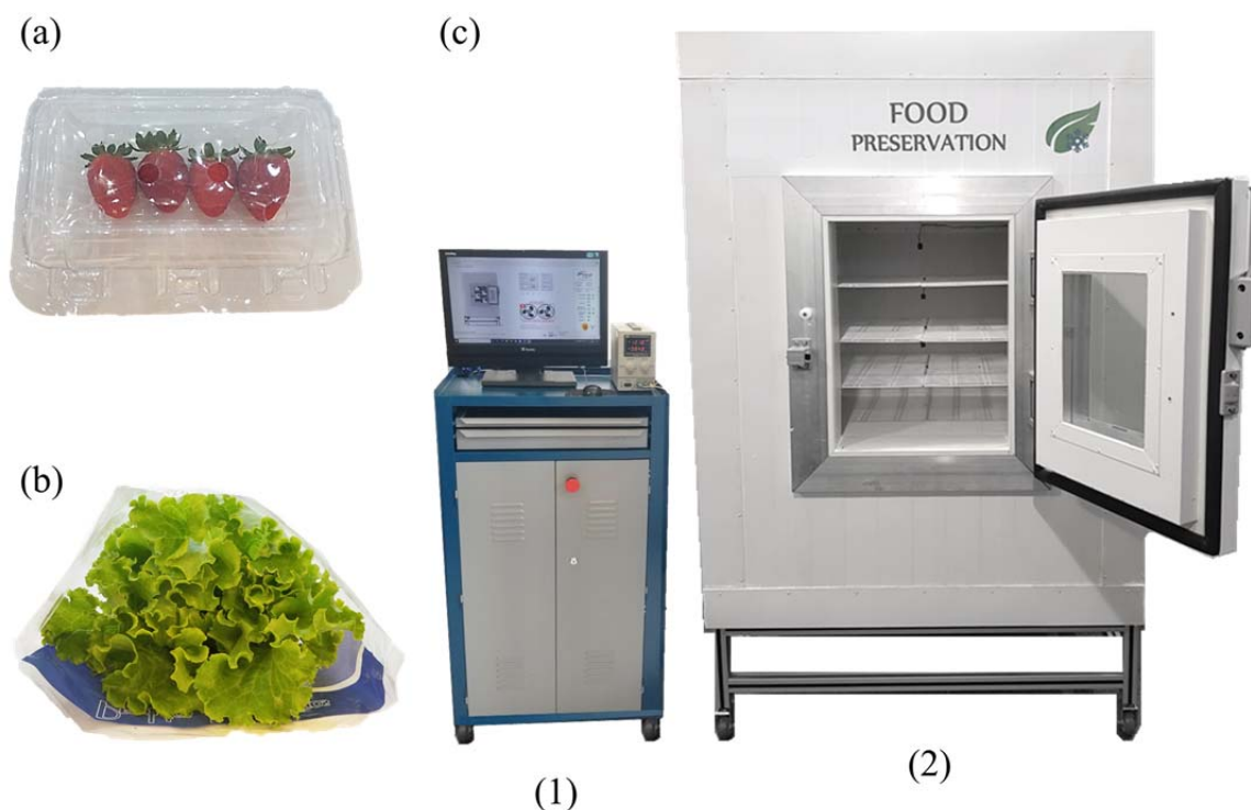
Figure 1: Packaged strawberry (a) and lettuce (b) samples for cold storage. Experimental facility (c) divided into a control unit (1) and the refrigeration system (2).
