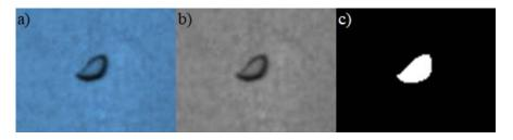
Figure 2: Selected stages of image processing; a) colour image, b) grayscale image, c) binary image
