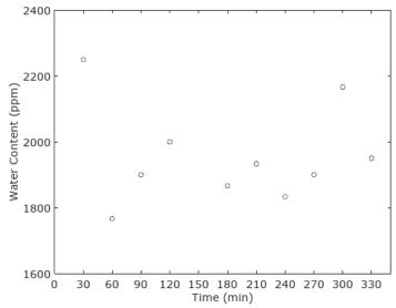
Figure 2: Outlet Water Content in Biodiesel for EXP1
