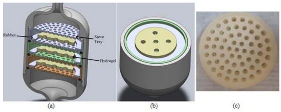
Figure 1: Bed Scheme for Removal of Water from Biodiesel. Internal (a) and External (b) views, (c) Sieve Tray
