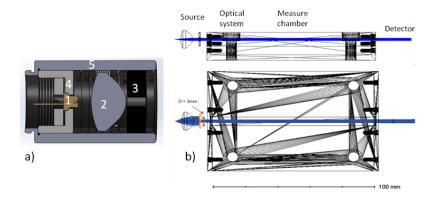
Figure 1: a) Optical system for laser source. 1 Laser diode, 2 Glass lens, 3 Shutter, 4 Mechanical support for laser diode, 5 Mechanical support for entire optical system. b) Optical simulation of laser beam, optical system, measure chamber and detector in Zemax.
