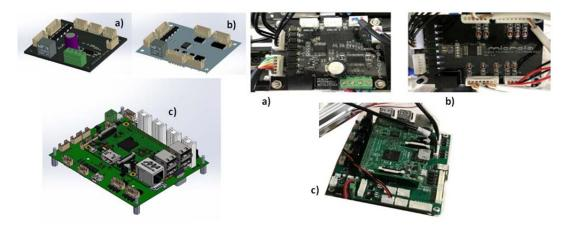
Figure 4: CAD renderings and realization of electronic boards: a) Moto-syringes board, b) valve board, c) motherboard.
