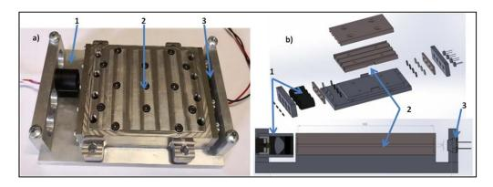
Figure 2: a) Final measure system manufactured. b) Explosion and section of the entire measure system. 1) Source 2) Measurement chamber 3) Detector
