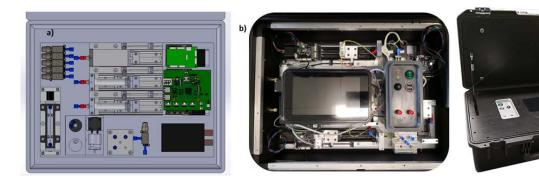
Figure 5: Portable device for Cr (VI) detection. a) Inside layout designed by Solidworks, b) Embedding in the portable carrying case, c) Final portable case.
