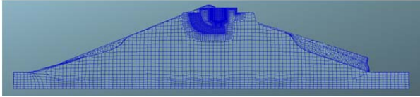
Figure 4. Numerical grid of the combustion chamber with spark plug placed in a central position.
