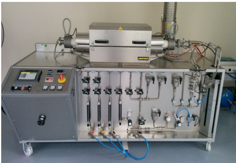
Figure 1: Nabertherm chemical vapor deposition furnace for impregnating carbon into CCC.
