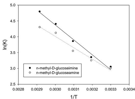
Figure 5: Arrhenius plot for N-methyl-D-glucosimine and N-methyl-D-glucosamine formation.
