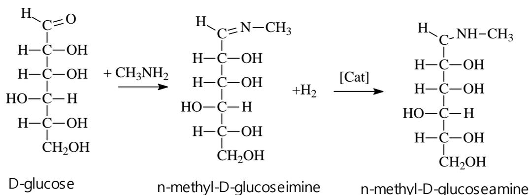
Figure 1: Scheme of N-methyl-D-glucosamine synthesis
