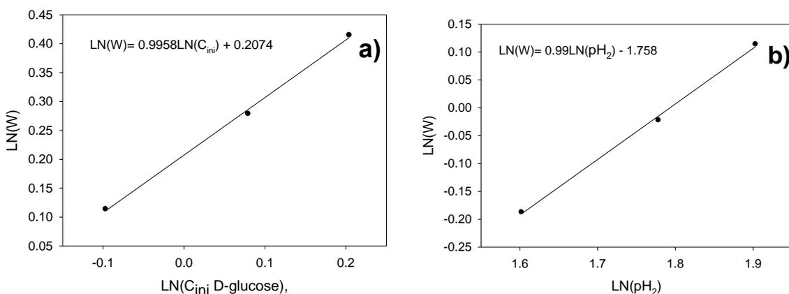
Figure 8: Determination of partial apparent reaction order for N-methyl-D-glucosamine synthesis for (a) D-glucose, (b) hydrogen.
