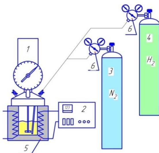
Figure 2: Reaction vessel for D-glucose transformation to N-methyl-D-glucosamine. 1 – Parr instrument high-pressure reactor, 2 – controller, 3 – tank for nitrogen, 4 – tank for hydrogen, 5 – heater, 6 – pressure reducer.
