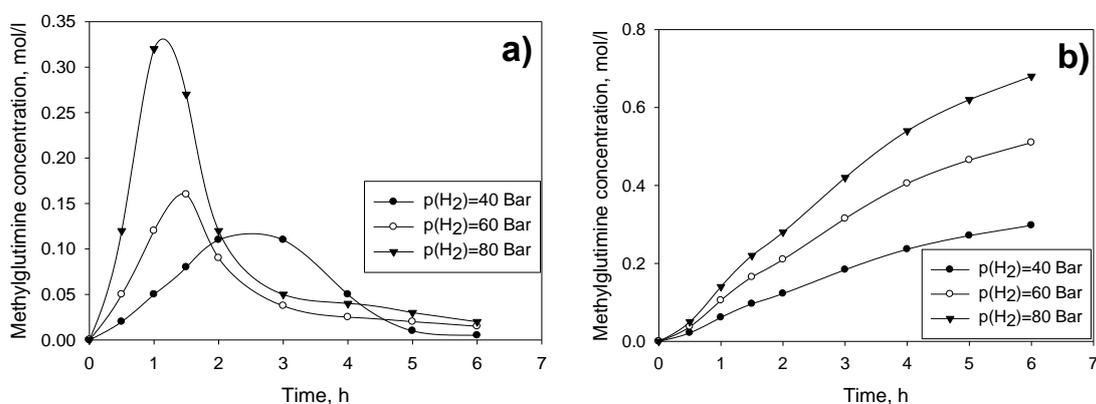
Figure 7: Hydrogen pressure influence on a) N-methyl-D-glucosimine, b) N-methyl-D-glucosamine yield.
