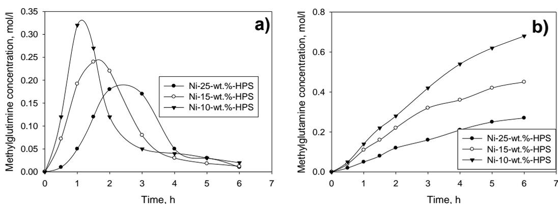
Figure 3: Investigation of synthesized catalysts activity for a) *N*-methyl-D-glucosimine, b) *N*-methyl-D-glucosamine yield.
