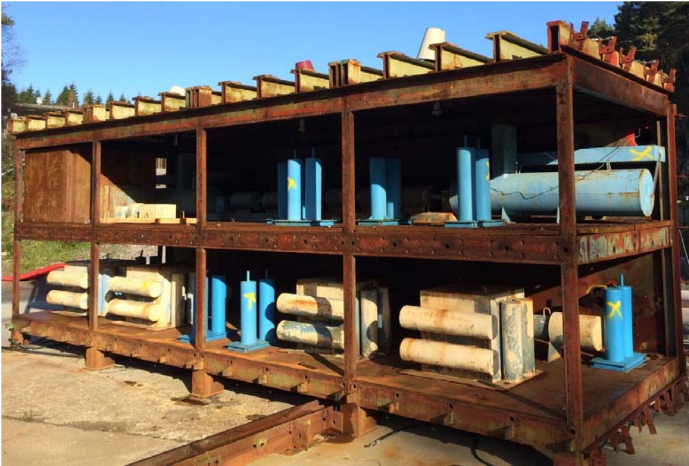
Figure 2: 50 m 3 explosion chamber used to investigate effect of aqueous of flame inhibitors
