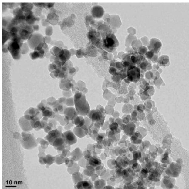
Fig. 2. The TEM micrograph of SiO<sub>2</sub> Nanoparticles.
