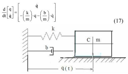
Fig. 1 Linearly damped harmonic oscillator
