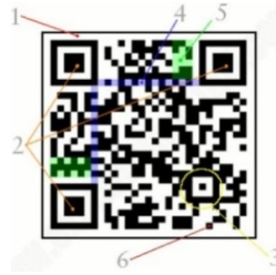
Figure 1. The six zones of a QRCode data (Ohbuchi, Eisaku & Lim, 2004)
