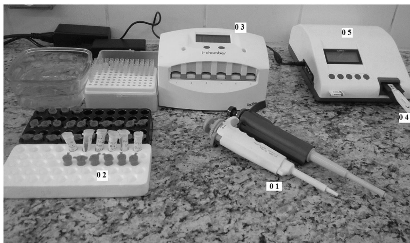
Figure 2. Cortisol analysis using the Ichroma Cortisol™ device, showing 30 µL and 75 µL pipettes (01), detection buffer tubes - orange color (02), incubator (03), sample loaded cassette (04), and scanner (05).
