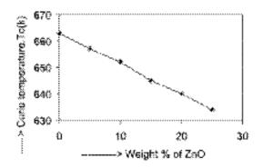
Fig. 2.6. Composition dependent Tc in Mn-Zn ferrite (Group B samples)
