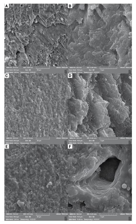
**Figure 2**. Representative SEM micrograms of the resin-dentin interfaces. A: G1, immersion in saline solution 0.9% for 30 minutes (control); B: Magnified image (10,000×) of (A); C: G2, immersion in CHX 2% for 30 minutes; D: Magnified image (10,000×) of (C); E: G3, immersion in NaOCI 5.25% for 30 minutes; F: Magnified image (10,000×) of (E).
