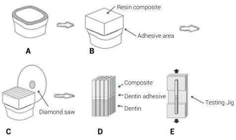
Figure 1. Sample preparation to micro- tensile bond strength test.
