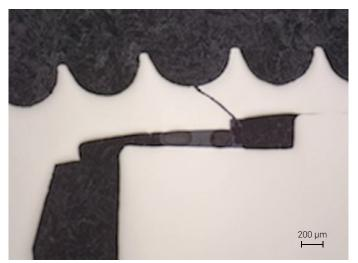
Figure 4. Optical microscopic evaluation: implant fracture at the discontinuity region of the abutment/ implant interface (approximated view). - FAC group.
