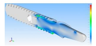
Figure 7. Finite element analysis of the FAC group implants: stress accumulation is represented in the red color located in the region with no contact of abutment/implant.
