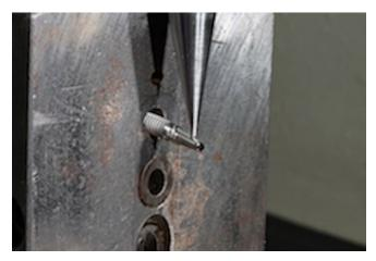
Figure 2. The implant and the metallic holder were fixed on the mechanical testing machine (EMIC; 2000DL) and submitted to a load cell of 500 KN capacity (KN500; EMIC).
