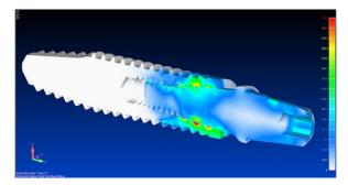
Figure 8. Finite element analysis of the CM group: stress accumulation is represented in the red color located in the region with no contact of abutment/implant.
