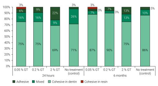
Figure 1. Bar diagram of the relative frequency (%) of failure modes, according to the concentration of the solution containing green tea extract applied to the dentin and the storage time.
