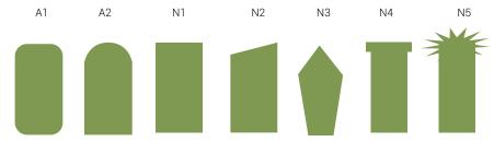
Figure 2. Classification of bristle tip morphology. Group A represents the acceptable rounding of the tip of the bristles, and group N represents the non-acceptable rounding of bristles tips.
