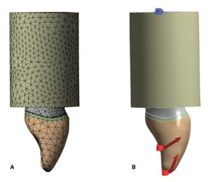
**Figure 4.** (A) Model with tetrahedral element of 0.8 mm. (B) Loading was performed in 2 steps: oblique load (135 degrees) of 100 N was applied to incisal third of lingual crown, and 25.5 N was applied perpendicularly to incisor crown.
