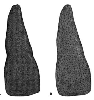
**Figure 2.** (A) Stereolithography triangulated (STL) file of incisor tooth obtained in InVesalius. (B) Incisor tooth STL file optimized for FEA using Mesh Prep Wizard within the CAD software SolidWorks.
