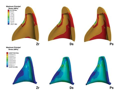
Figure 5. (A) Maximum Principal Stress in ceramic veneer and (B) Maximum Principal Strain in core of Zr, Ds and Ps groups, respectively.
