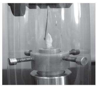
Fig. 1. Shear strength testing in the Instron machine.
