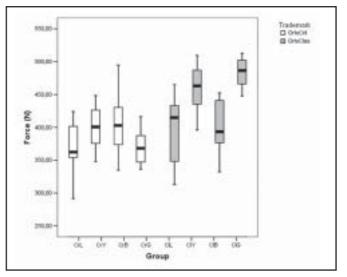
Figure 3 - Box Plot comparing trademarks and colours of acrylic resins. Mean, SD, max, min.
