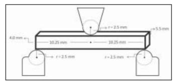
Figure 2 - Flexural strength test schematic's representation.
