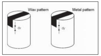
Fig. 1. Dimensional accuracy of a cast crown expressed by the discrepancy measured on its was pattern (dx) and coating (dy) on the same die.
