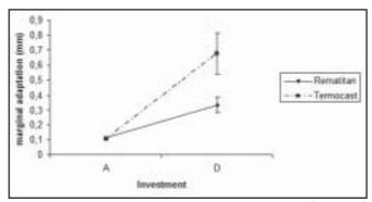
Fig. 2. Marginal discrepancies of the cast MOD titanium inlays invested with Rematitan Plus<sup>\*</sup> and Termocast<sup>\*</sup>. Each line represents the means and standard deviation before (A) and after (B) casting.
