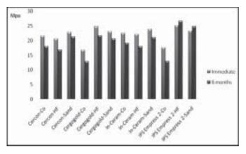
Fig 1. Shear bond strength (MPa) of ceramics in accordance with surface treatment and storage time.
