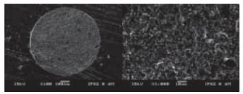
Fig 2. SEM of IPS Empress 2: Cohesive fracture pattern (arrow) (A- Original magnification X 100; B-Original magnification X 1000).
