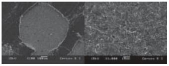
Fig 5. (a) SEM of Cercon: Adhesive fracture pattern (arrow) (A- Original magnification X 100; B- Original magnification X 1000).
